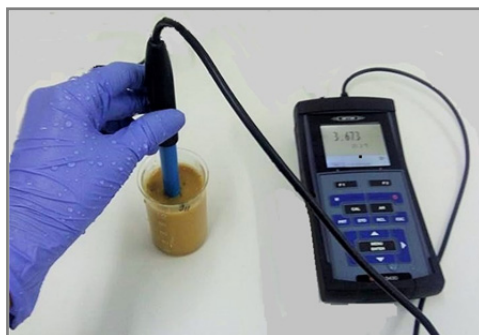
Fig. 2. The Determination of pH in laboratory
