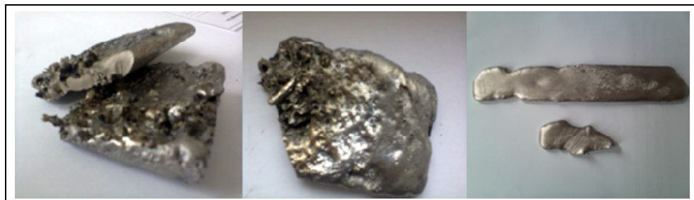
Fig. 6. Multi-component alloy ingots resulting from the melting of WEEE in a microwave field
