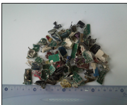
Fig. 5. Grinded electric and electronic equipment wastes
