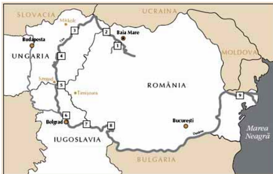
Fig. 2. The course of toxic substances from the Aurul Bozânta Mare tailing pond, Maramureș County (1 - cyanide discharge from the tailing pond; 2 - cyanide wave reaches the Romanian - Hungarian border; 3 - Tiszalok, Hungary; 4 - Szolnok, Hungary; 5 - Hungarian - Yugoslavian border; 6 - Beograd (Perlez), Yugoslavia; 7 - Drobeta Turnu-Severin, Romania; 8 - Porțile de Fier, Romania; 9 - Danube Delta, Romania) (UNEP).
