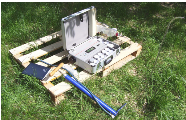
Fig. 2. The LUK3C detector and accessories for radon concentration measurement in soil gas.
