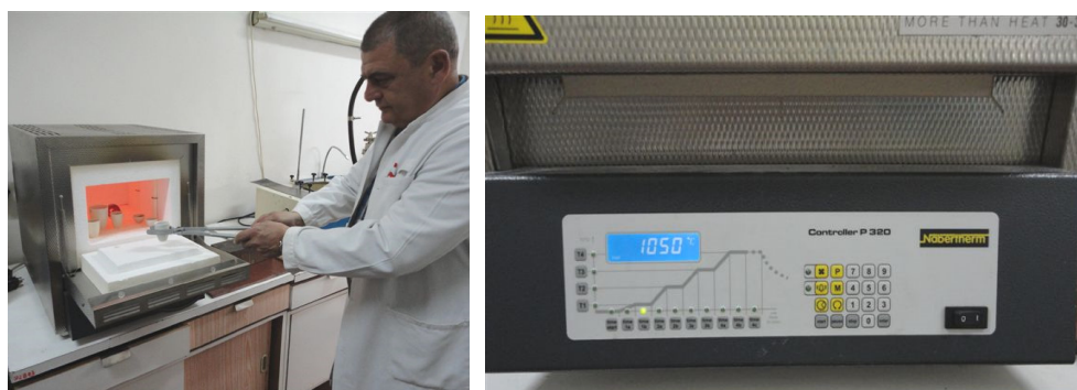
Fig. 2. Calcination of asbestos cement samples in the Nabertherm Controller P320 furnace
