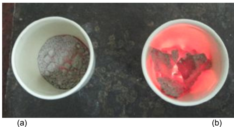
Fig. 3. Asbestos cement samples after calcination: a) ground sample; b) crushed sample.
