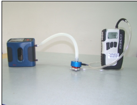
Fig. 3. Pump connected with PEM and flow meter
