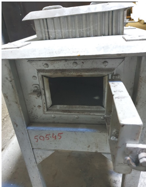
Figure 9. Handmade electric oven with resistors
