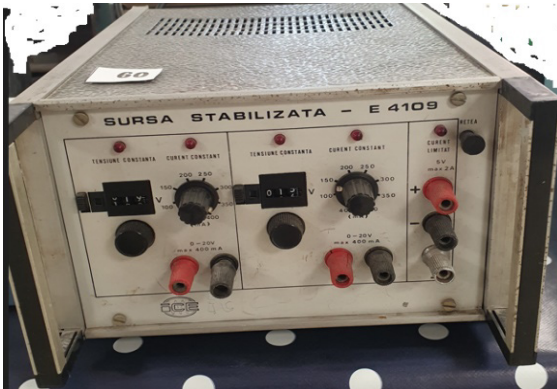
Figures 11. E-4109 triple stabilized DC power supply with short circuit protection
