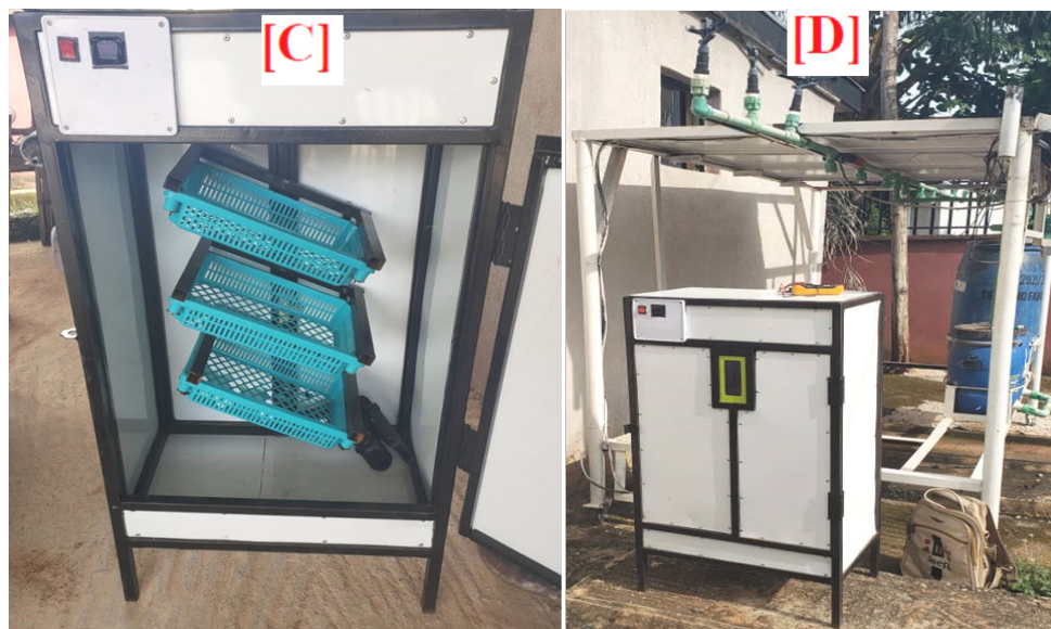
Plate 1. Arrangement of incubator skeleton (a), assemble of incubator members (b), rotating egg tray inside incubating chamber (c), and completed solar-powered incubator connected to the solar power
