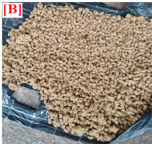
Plate 2. Freshly produced pellet-mash at 27.1% moisture content (a) and oven-dried pellet-mash at 15.1% moisture content (b).
