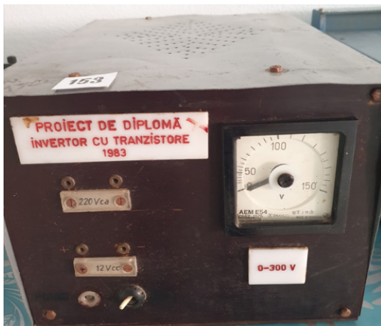
Figures 15. Inverter with transistors. The practical implementation of a Diploma Thesis from 1983
