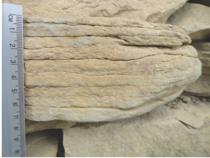
Fig. 2. Severe delamination along the bedding planes.
