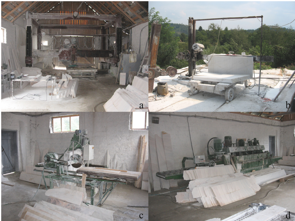
Fig. 6. Marble processing equipment (a. circular sawmill; b. blade sawmill; c. circular saw; d. grinding and polishing machine)
