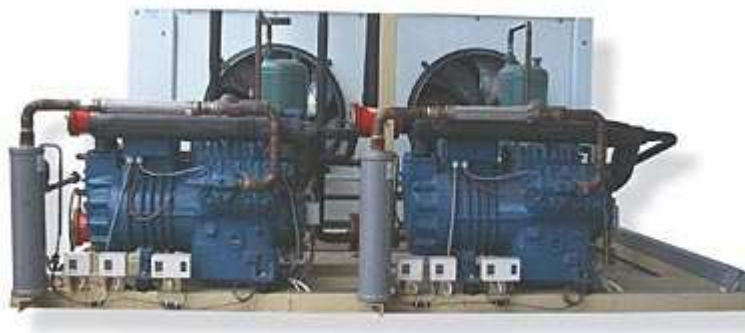
Fig. 5. The refrigerating plant, noise source
