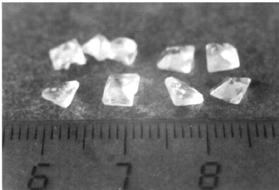
Fig. 1. \text{La}_2(\text{SO}_4)_3 \cdot 9\text{H}_2\text{O} single crystals grown from solution by the slow evaporation method.
