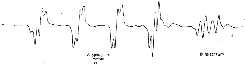
Fig 1 ESR spectrum of KDP Cu 2+ crystals recorded for a H || c direction
